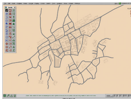
Correlated terrain output generated by Terra Vista for JSAF.
